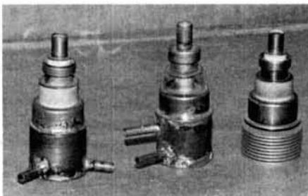
Three 2C39 tubes include an unmodified tube (right) with original finned heat sink in place. Tube on left is from early T44 (plunger tuning) and tube in center shows "dry run" or first try at modification. Note slightly different placement of water inlet and outlet tubes.
